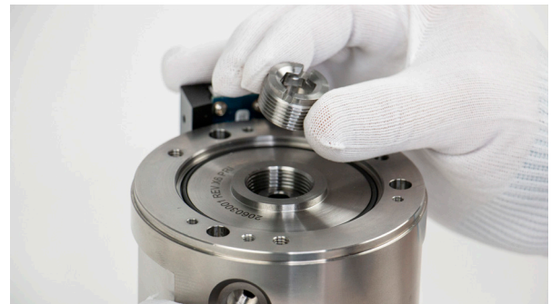
Figure 8.1.2.2.1-E Removing the cylinder jam nut
