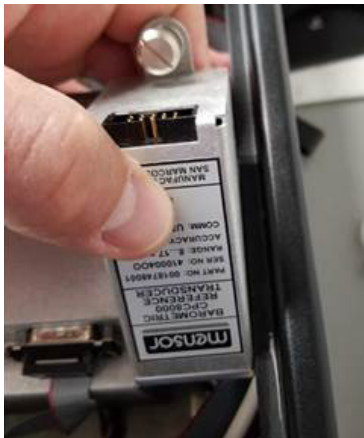
Figure 8.1.3.5-B Barometric Reference Removal
