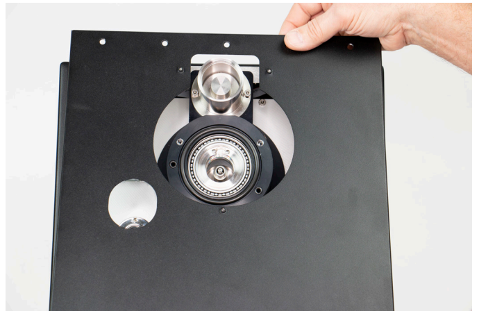
Figure 8.1.3.4-B Top Cover Removal
