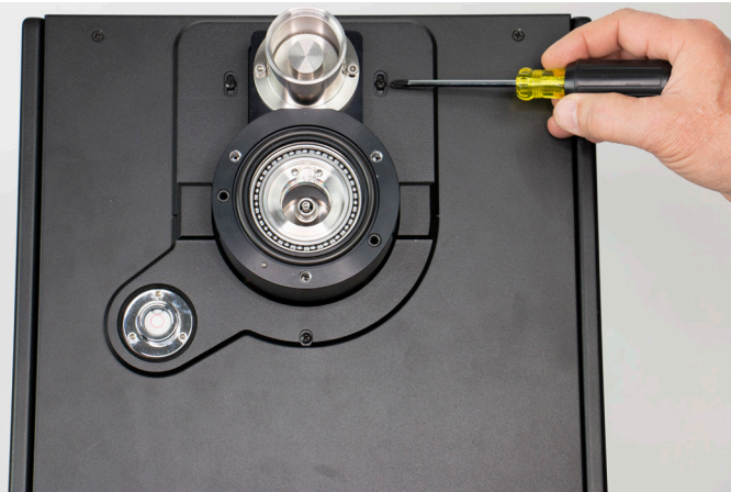
Figure 8.1.3.4-A Trim Plate Removal
