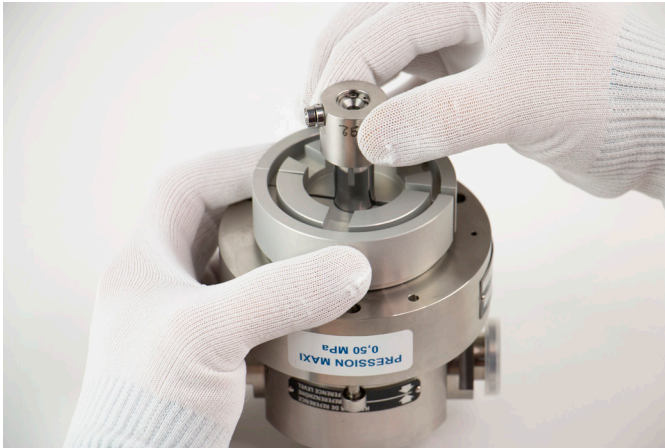
Figure 8.1.2.1.3 Measuring Head Reassembly
