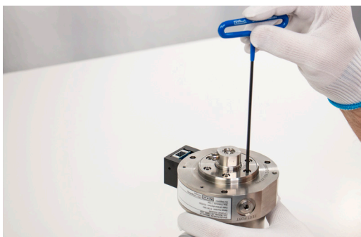
Figure 8.1.2.1.1-A Removing retaining ring
