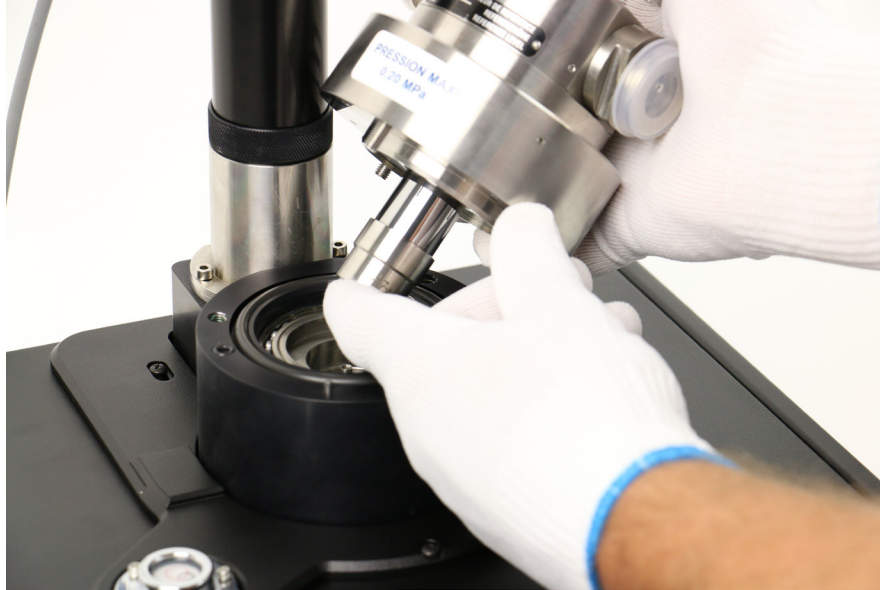
Figure 5.4.2-E Legacy 610 aligning with base
