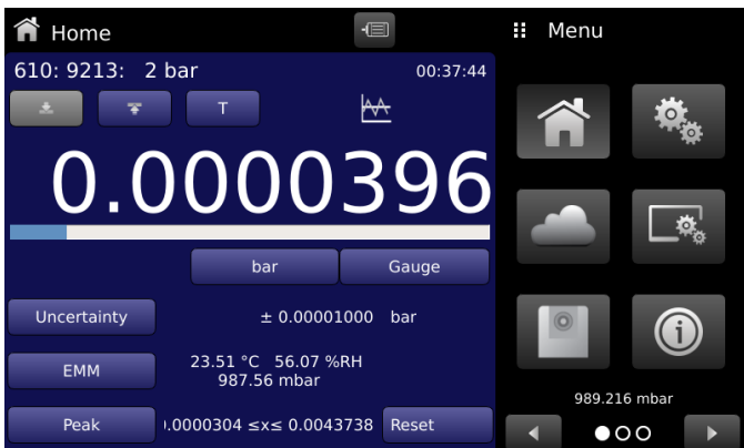
Figure 6.4.1.1-B Unstable Pressure Reading
