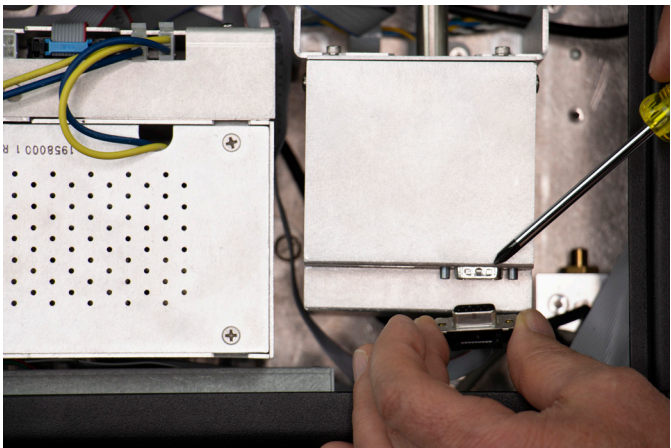
Figure 8.1.3.4-C Unplugging Vacuum Transducer
