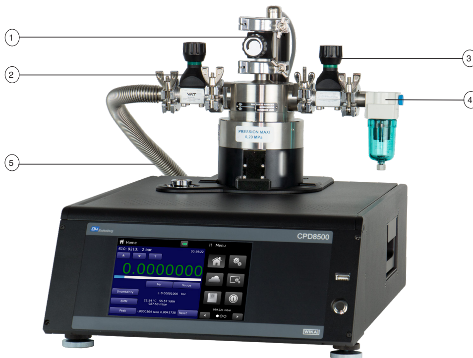
Figure 5.7.3 Low Pressure Absolute Pressure Connections
