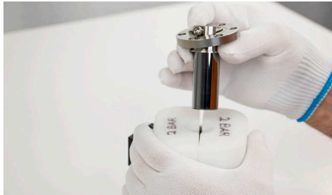
Figure 8.1.2.1.1-C Removing the piston
