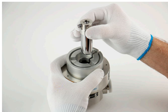
Figure 8.1.2.1.1-A Removing The Piston From Head
