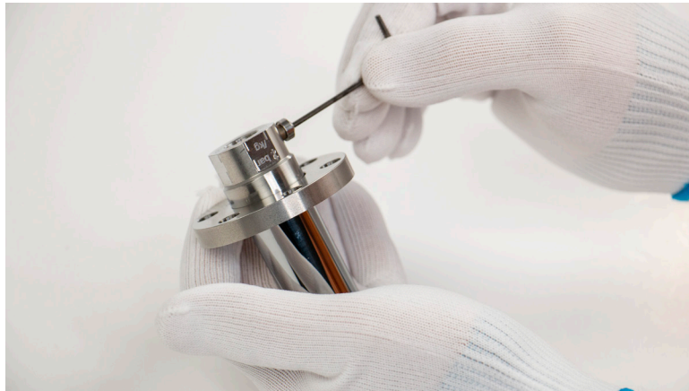
Figure 8.1.2.1.2-B Removing piston retaining ring
