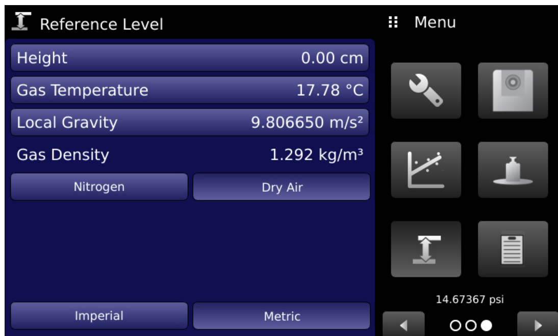
Figure 8.2.9 Reference Level App (Dry Air)
