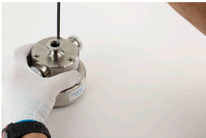
Figure 8.1.2.1.1-B Removing Top Cap
