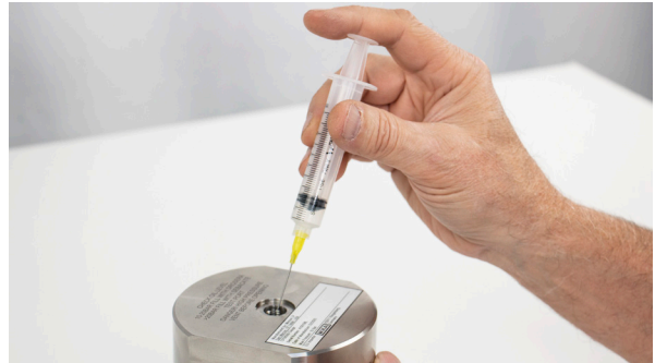
Figure 8.1.2.2.2-D Fill with oil
