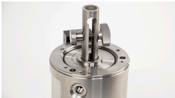
Figure 8.1.2.2.1-F Removing the cylinder
