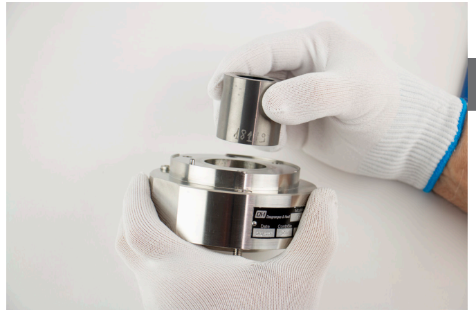
Figure 8.1.2.1.1-D Removing Cylinder From Head
