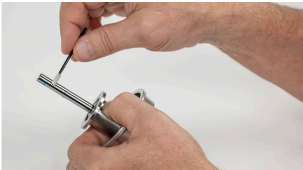
Figure 8.1.2.2.2-C Swab piston with oil
