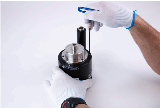
Figure 8.1.2.2.1-A Separating Measuring Head
