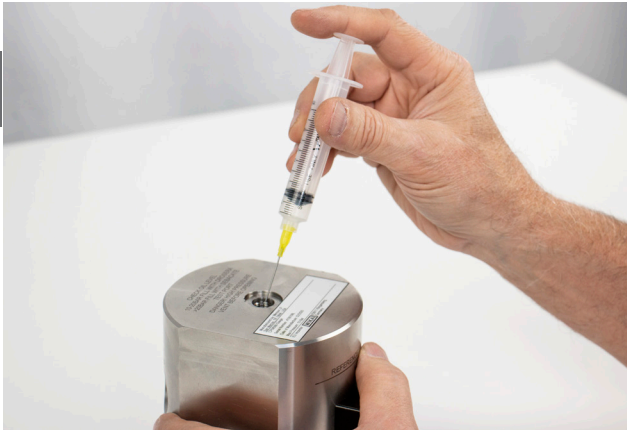
Figure 5.4.2-F Adding Oil to the Gauge Head
