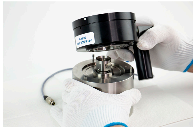
Figure 8.1.2.3.1-A Separating Measuring Head
