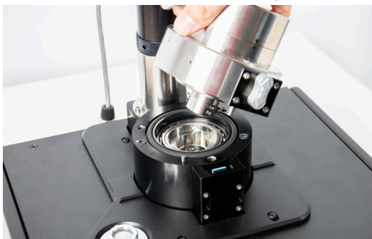
Figure 5.4.1-G Aligning the CPS8500A
