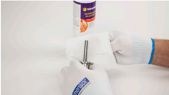
Figure 8.1.2.2.2-A Cleaning the piston and cylinder
