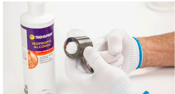
Figure 8.1.2.1.2-A Piston and cylinder cleaning
