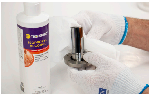
Figure 8.1.2.1.2-A Piston and cylinder cleaning
