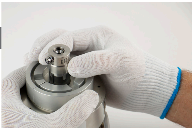
Figure 8.1.2.1.1-A Removing The Piston From Head
