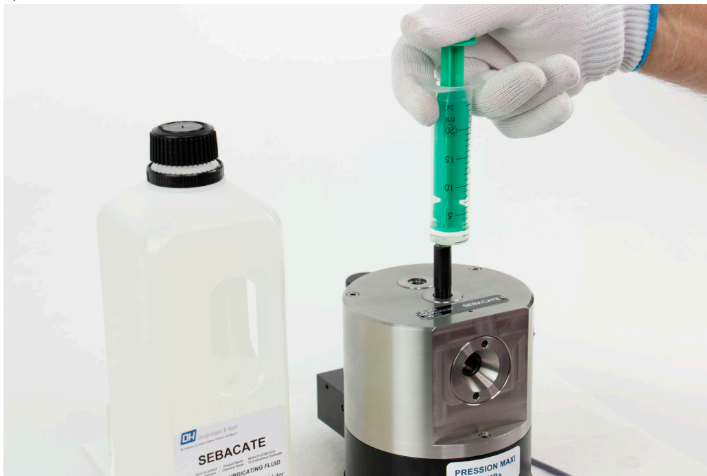
Figure 8.1.2.3.3-A Oil Filling Process
