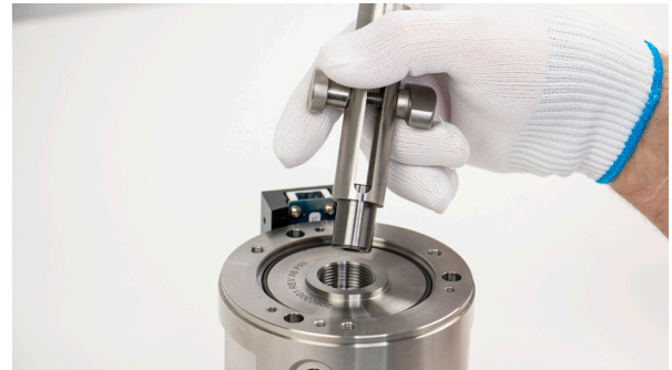
Figure 8.1.2.2.1-F Removing the cylinder
