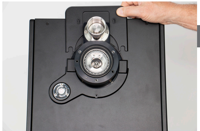
Figure 8.1.3.4-A Trim Plate Removal
