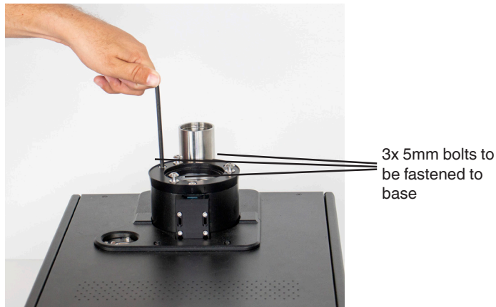
Fig 5.8.2-B Install gauge adapter
