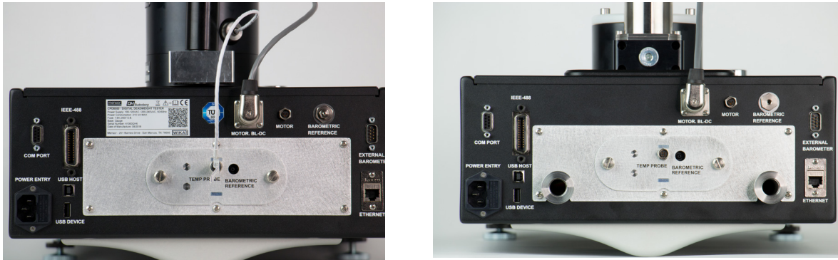
Figure 5.10-A Rear Panel - Gauge (left) and Absolute (right)
