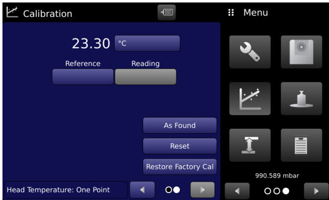
Figure 8.2.6.1-A One Point Calibration (As Found)
