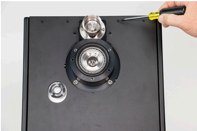
Figure 8.1.3.4-B Top Cover Removal
