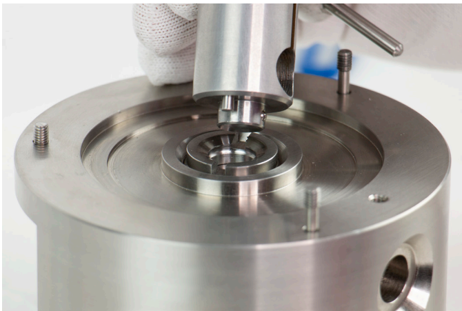
Figure 8.1.2.3.1-C Jam Nut Removal
