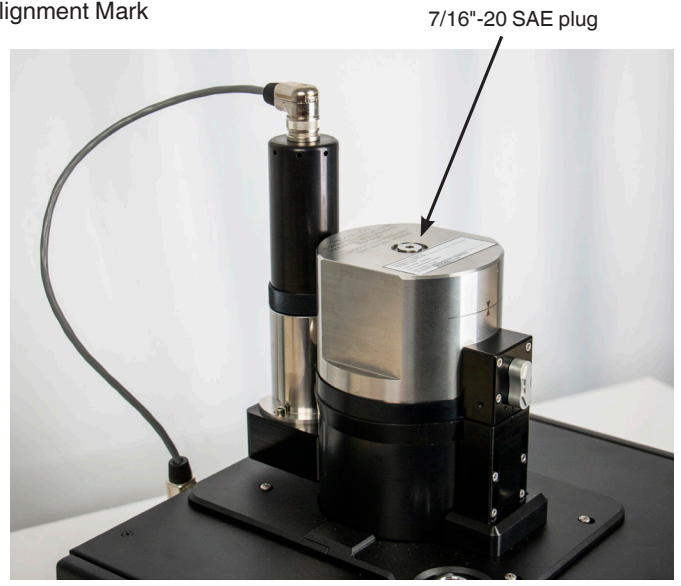
Figure 5.4.2-E Securing the Head
