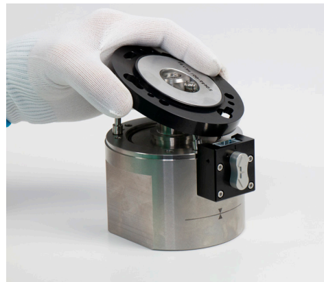
Figure 8.1.2.2.1-B Removing Bayonet Ring
