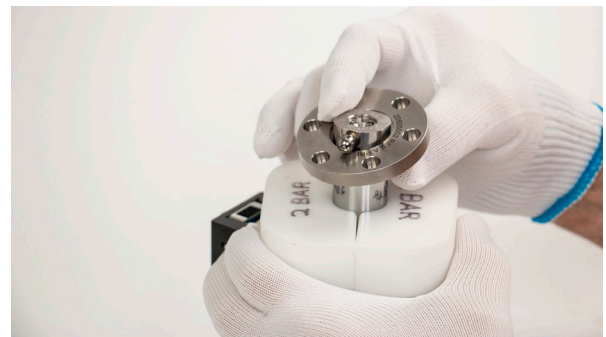
Figure 8.1.2.1.1-B Piston removal tool
